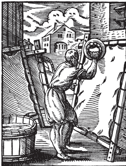
Figure P1.4 Parchment—Scraping and smoothing animal skins is part of the ancient process of preparing parchment, a long-lasting but expensive medium. Woodcut by Jost Amman (1539–91) from “True Description of all Professions on Earth, exalted and humble, spiritual and worldly,” 1568.
